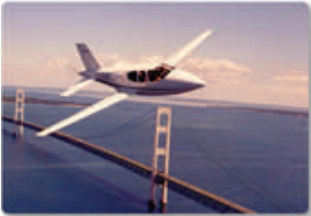
We first developed the SR20, a four-passenger, single-engine composite aircraft that was awarded FAA Type Certification in 1998. It incorporates flat-panel, multi-function display technology and state-of-the-art safety innovations, including a final level of protection known as the Cirrus Airframe Parachute System™ (CAPS).
