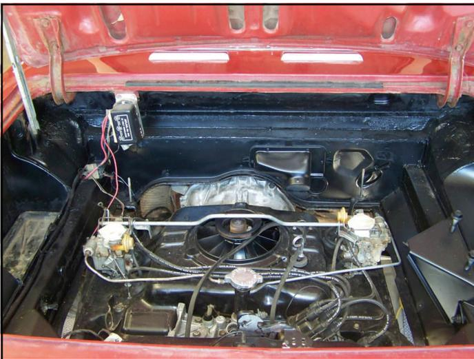
Here's a couple of pictures of Art's 64 engine going back in. After a 2nd trip up to his garage with all the needed bolts and parts it went in like a dream. We had to pull the starter off and clean all the connections and then she fired right off. Now for some exhaust and a front perimeter seal and she'll be ready to go. He needs some brake work and a few other things done before she hits the road. It's coming along good.
