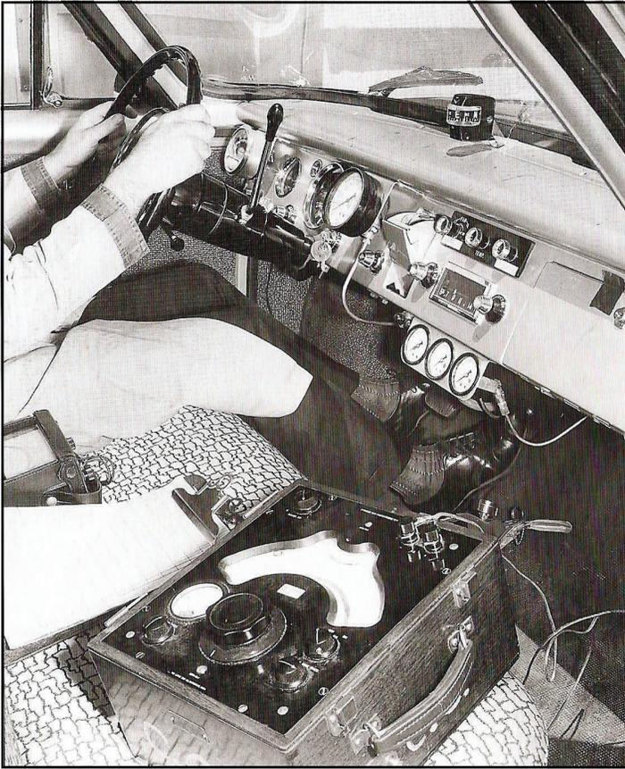
A look inside the cockpit of a Corvair "Holden Special" prototype revealed a wide range of test instrumentation for this automatic-transmission car. It's gear selector was column-mounted. The large test apparatus in the foreground was connected as needed to thermocouples in the engine room and elsewhere to measure component temperatures.
